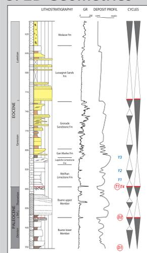
Fig. 5 : Synthetic log and stratigraphical interpretation of well core data.
