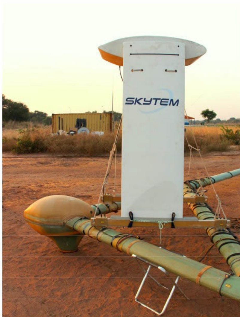
Figure 3 Rudder containing the Z coil located in the top part of the tower.
